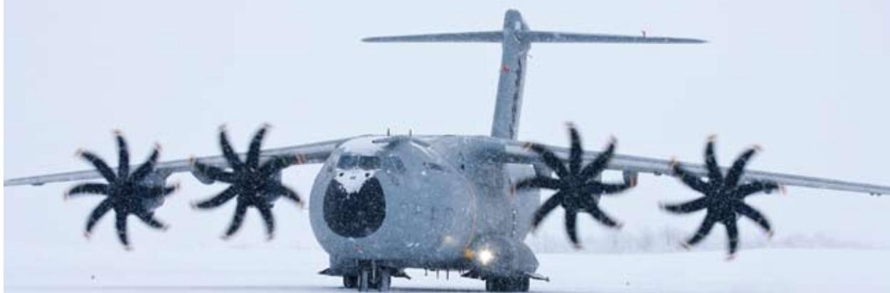
*ABOVE: The Second Airbus Military A400M development aircraft spent four days in Kiruna, northern Sweden, for cold weather trials in February. Temperatures down to -21 degrees C were experienced and the aircraft successfully achieved all the planned test points during a programme that focused on the performance of the powerplants. (Airbus Military photo)*
