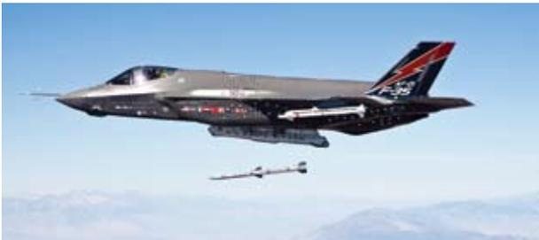
*ABOVE - A recent image of test aircraft AF-1 dropping an AIM-120 AMRAAM in separation tests over the China Lake test range in the USA. The same aircraft has also dropped a 2,000lb GBU-31 bomb from its internal weapons bay. (LM photo)*
