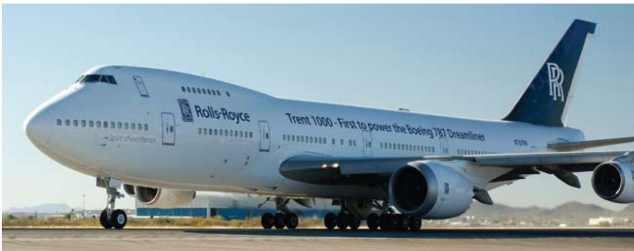
ABOVE - Rolls-Royce recently completed the first flight tests on a Boeing 747-200 of the latest updated version of the Trent 1000 for the Boeing 787-9. This engine can provide 74,000 lbs of thrust, which will be well matched to the stretched 787. (Rolls-Royce photo)
