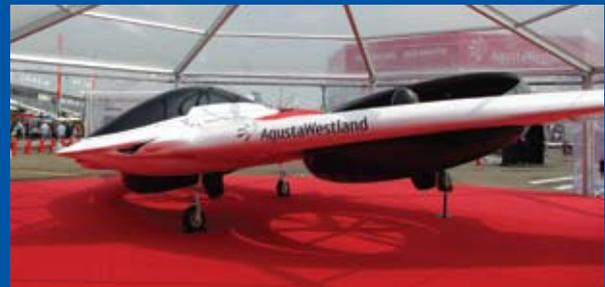
*ABOVE - The Project Zero electrically-driven tilt lift fan concept demonstrator from AgustaWestland, which was displayed in public for the first time at the Paris air show, will lead to new concepts adaptable to helicopter use as well as advancing experience of highly innovative VTO technologies for the future.*
