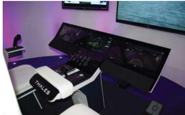
ABOVE: The cockpit of the future – the latest Thales integrated touch-screen cockpit design is fully interactive and enables pilots to select displays showing as much, or as little, as they need, day or night in all weathers, from airport taxiing instructions to route flying and global airport approaches with real-time sensor imagery overlaid on 3-D terrain and obstacle representation.
