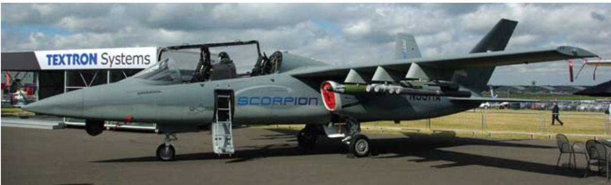
ABOVE: Involving no US government funding, the prototype Textron AirLand Scorpion, built largely from composite materials, and off-the-shelf systems and components, flew after only 18 months from project go-ahead. It was exhibited at Fairford and Farnborough with a range of potential attack weapons, showing its potential as a low cost replacement close support aircraft for such aircraft as the A10 or armed Hawk or Tucano.
