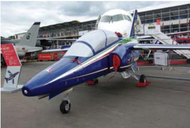
ABOVE - The global fight for new trainer orders continues, and within the Finmeccanica static park at Farnborough were examples of the familiar M-346 advanced trainer and the re-launched M-345 HET, a lightweight single powered trainer offered as a replacement for older turboprops and light jets.
